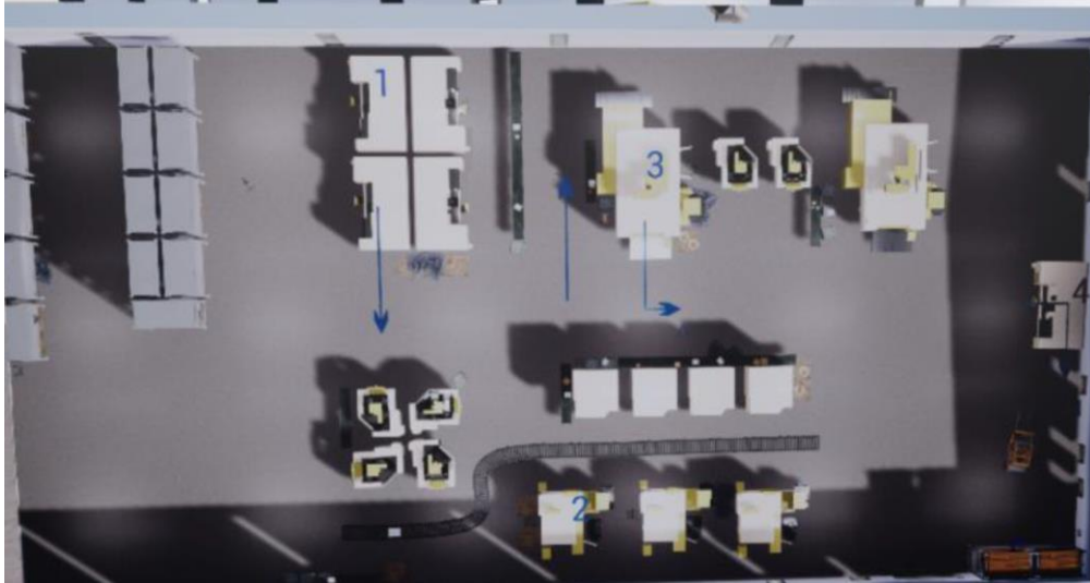
Figure 7. A top view of the final solution to visualize flows in the factory. Blue numbers for the order in which the machines should be accessed, pulsating and moving blue arrows between. A
