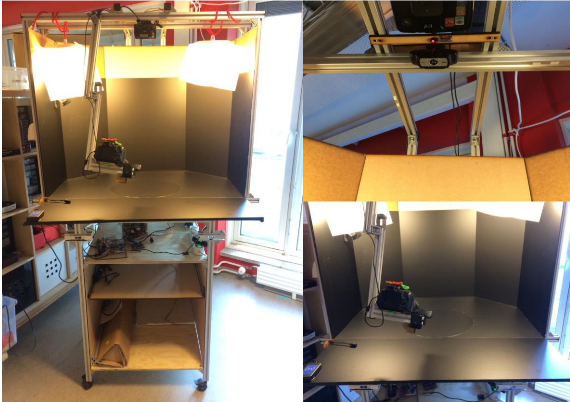
Figure 1. The Protoboost used for testing new features. The camera used for detecting and capturing sketches is shown on the top right image.
