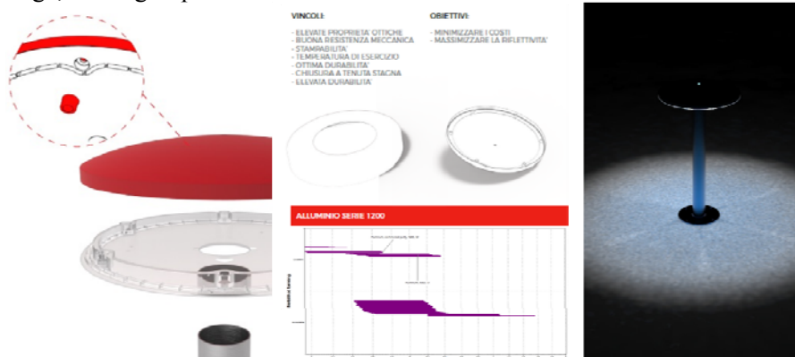
Figure 4. Workshop (A) - Innovation by the change of the light diffuser shape and material
