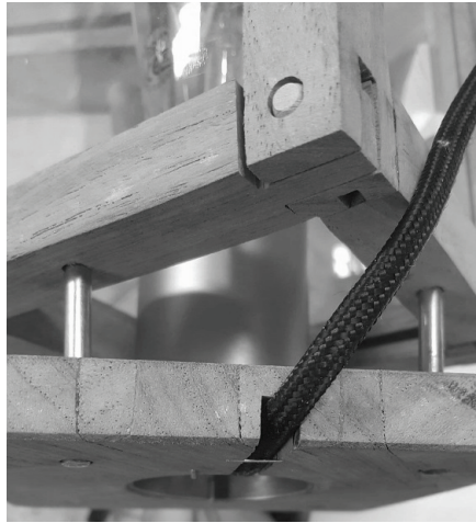
Figure 1. The bottom of the lamp is joined with several bits of wood and the base for the lightbulb is inserted in the bottom. Tracks for the cord are carved, and the plugs are old, golden steel pipes cut with a hacksaw.
