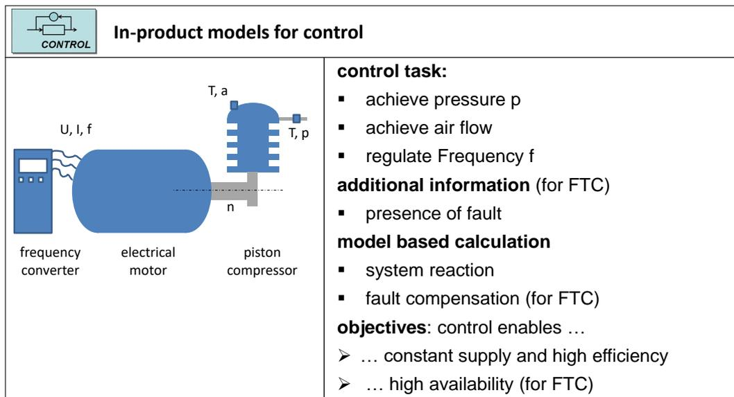
Figure 5. In-product model for control: example
