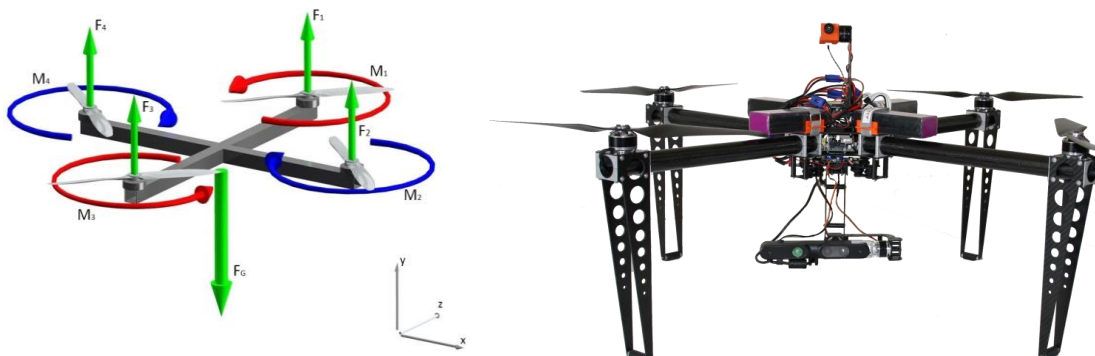
Figure 1. Left: Basic structure of a multicopter; right: realized multicopter
