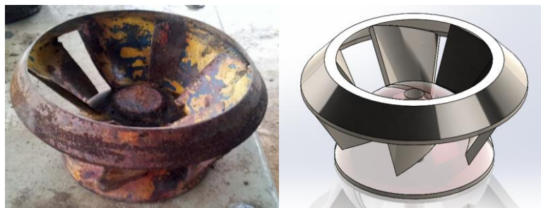
Figure 3. Impeller sample (left) and CAD model (right) of TmIP
