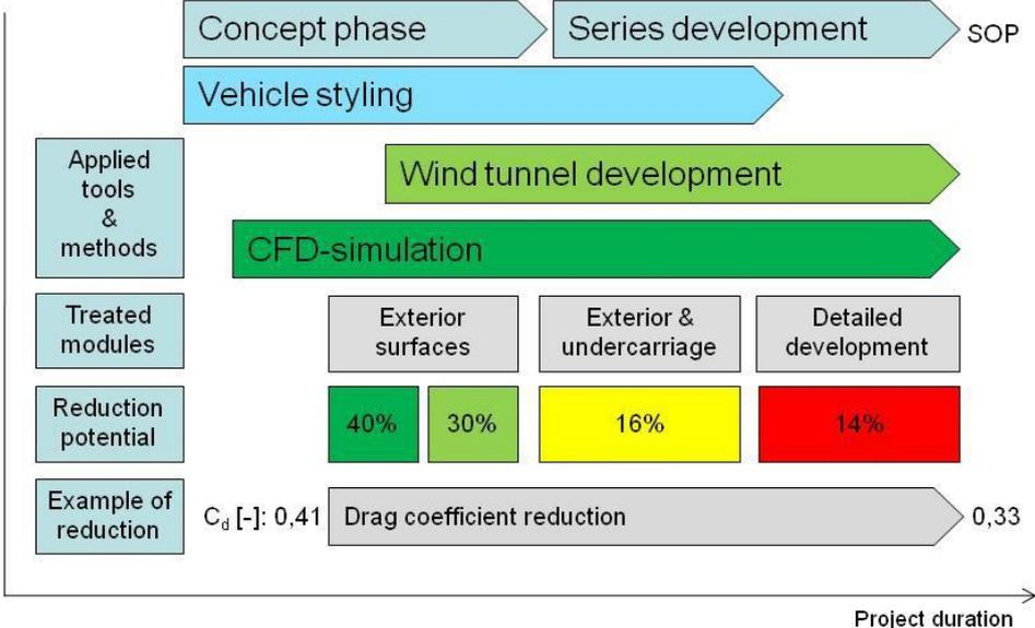
Figure 2: Exemplary workflow of aerodynamic investigations in automotive development, according to [4]
