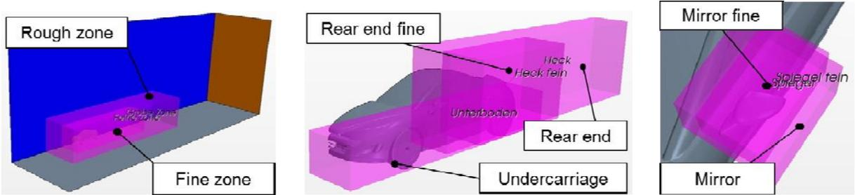
Figure 6: Examples of local mesh refinement areas of the start-up file for CFD [8]
