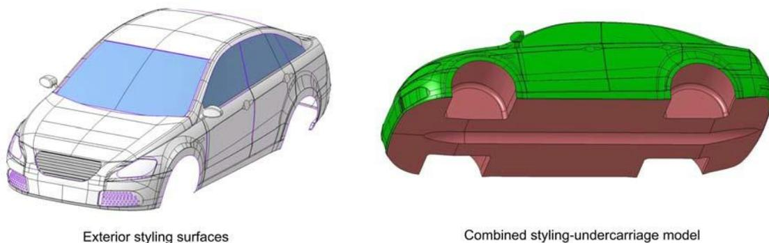
Figure 3: Example of exterior styling surfaces and a conceptual combined styling-undercarriage model
