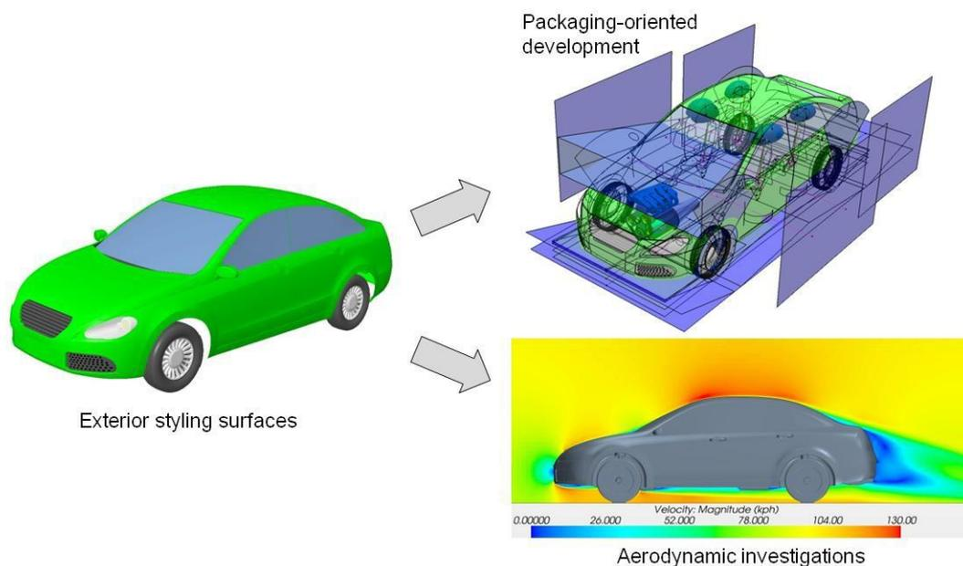
Figure 1: Exterior styling data as a basis for packaging-oriented development and aerodynamic investigations
