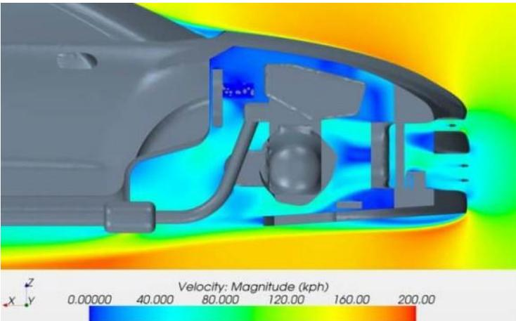
Figure 7: Engine compartment flow [8]
