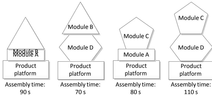
Figure 1. Example of product assembly times depending on combinations of modules
