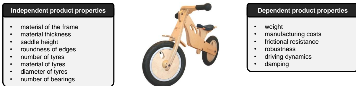
Figure 5. Product properties using the example of a wooden balance bike (picture credits by Lloyds Worcester Ltd, 2014)
