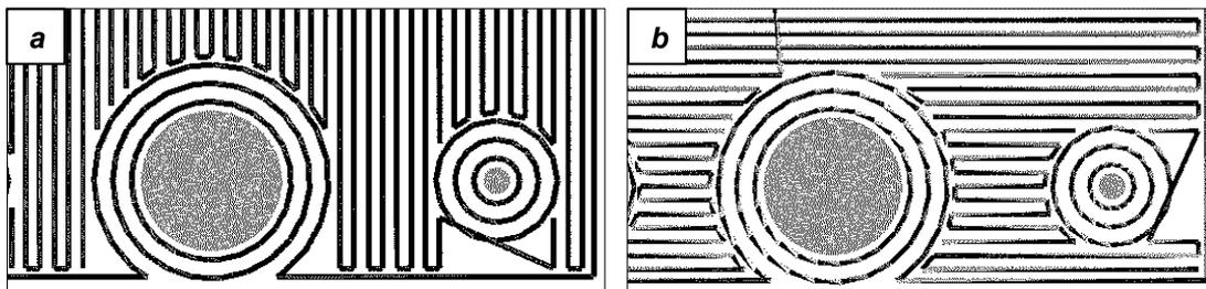
Figure 12. Top layers alternate between  $0^\circ$  and  $90^\circ$  a) top layer b) successive layer
