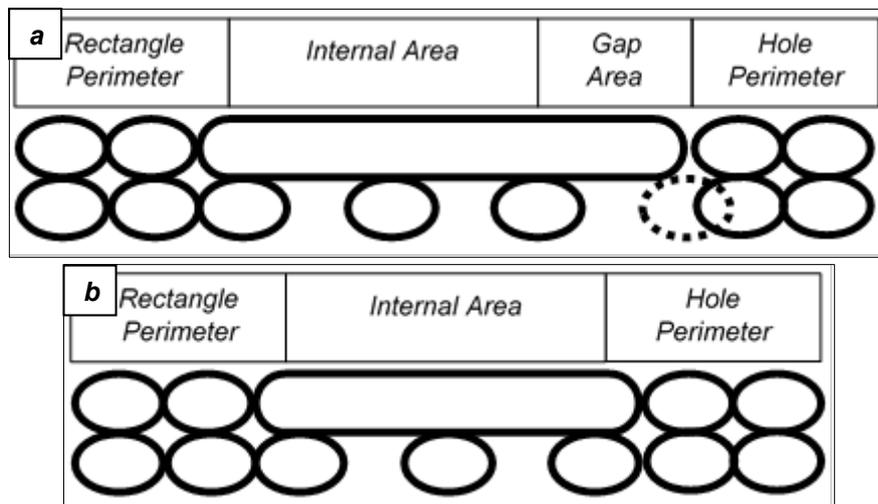
Figure 14. a) Sketch of cross-sectional area showing how the perimeter roads prevent placement of additional fill road. The dotted ellipse shows where a fill road should go for the pattern to repeat fully b) Sketch of a cross-sectional optimized for the Dimension printer
