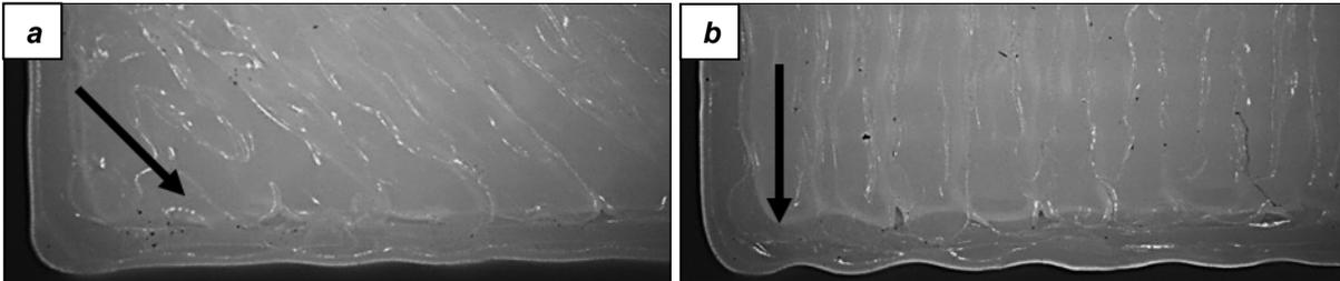
Figure 1. Top views of the printed parts: a) part printed vertically b) part built at 45° offset
