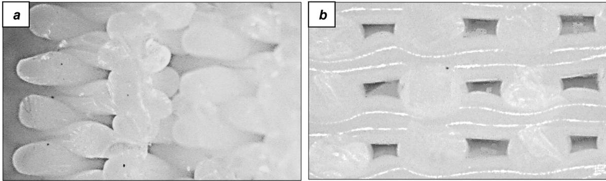
Figure 3. Cross-sections of parts along the length of the rectangle a) part with alternating 45 and 135° deposition paths shows crossed ends b) part with alternating 0 and 90° deposition paths shows grid-like structure
