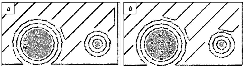
Figure 9. Cubify middle layers at  $45^\circ$  do not alternate deposition angles between layers a) a middle layer b) successive middle layer
