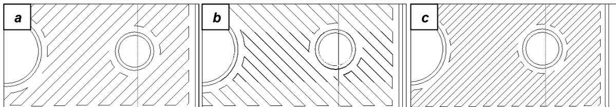
Figure 8. StratasysEX layers alternate between  $45^\circ$  and  $135^\circ$ : a) middle layer orientation b) successive layer c) Top layer with closer spacing between deposition paths
