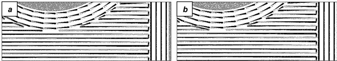
Figure 11. Bottom layers do not alternate deposition angles a) bottom layer b) 2<sup>nd</sup> layer
