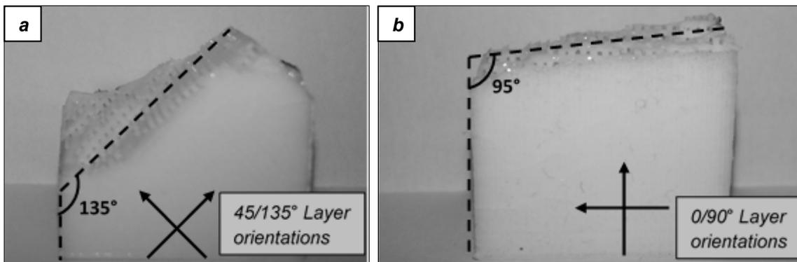
Figure 2. a) part with alternating 45 and 135° deposition paths shows a diagonal fracture plane b) part with alternating 0 and 90° deposition paths shows a horizontal fracture plane
