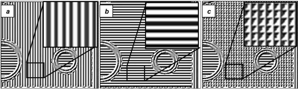
Figure 10. Makerbot Desktop layers alternate between  $0^\circ$  and  $90^\circ$  with only one exception:
