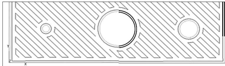
Figure 5. StratsysEX showing 2 outer paths around block and hole perimeters. The darkened lines indicate the 2 paths that become the surfaces of the part.
