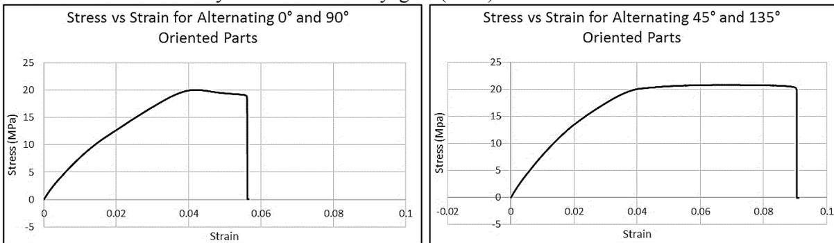
Figure 15. Stress vs Strain graphs from tensile testing on rectangular coupons
