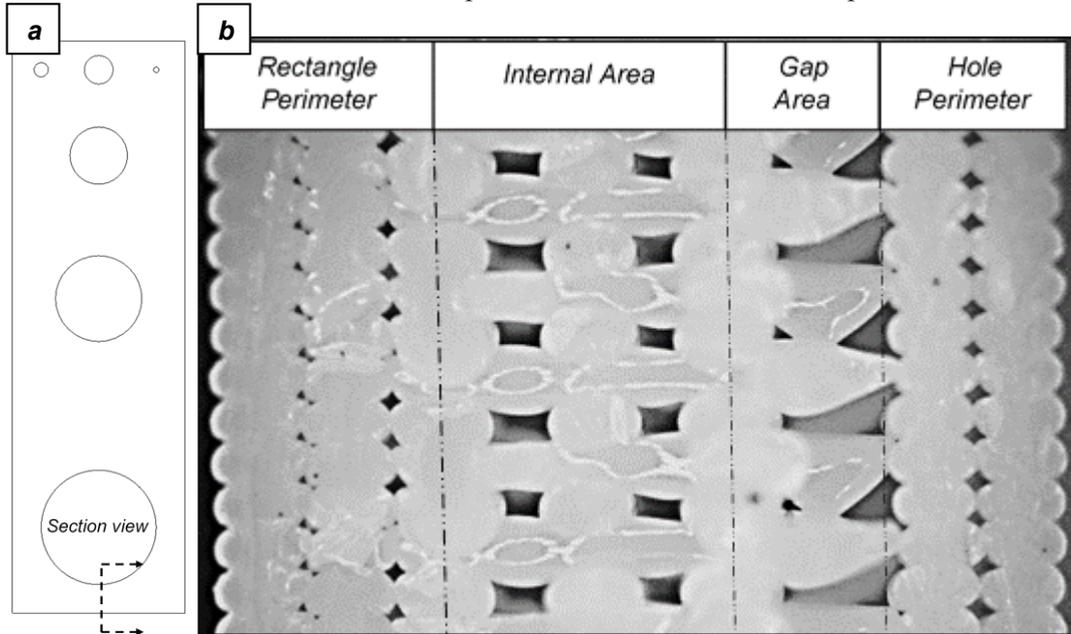
Figure 13. Cross-sectional area across the section between the outside perimeter (left) and the largest hole perimeter (right). On the right, the Gap Area shows the area where there is minimal adhesion between the fill roads and the hole perimeter roads
