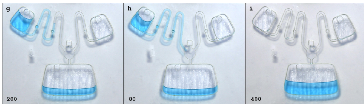
Figure 7. Capture of the left fluid first crossing the second capillary valve, then the second siphon valve and finally flowing into the big reservoir
