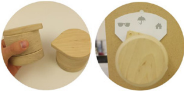
Figure 3: The objects are connected to Internet by wifi, but have an exterior totally made out of wood. To the right as connected devices, where turning the bottom knob on one of the objects the other's head start to turn in a 1:1 relation. To the left as an information display.
