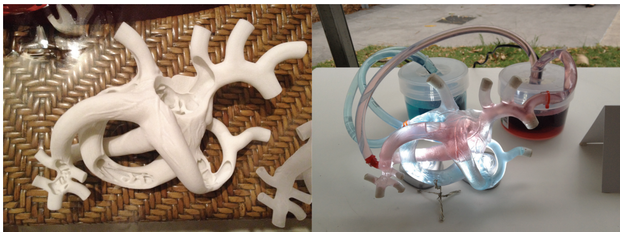
Figure 3. Heart provocation models by MA student Kaecee Fitzgerald (a) 3D print from the CAD model; and (b) 'Double pump' heart in action showing flow
