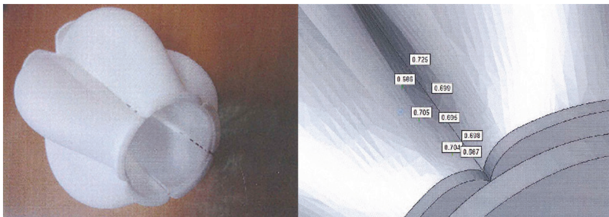
Figure 2. Print failure report from Shapeways showing insufficient wall thickness in the seams
