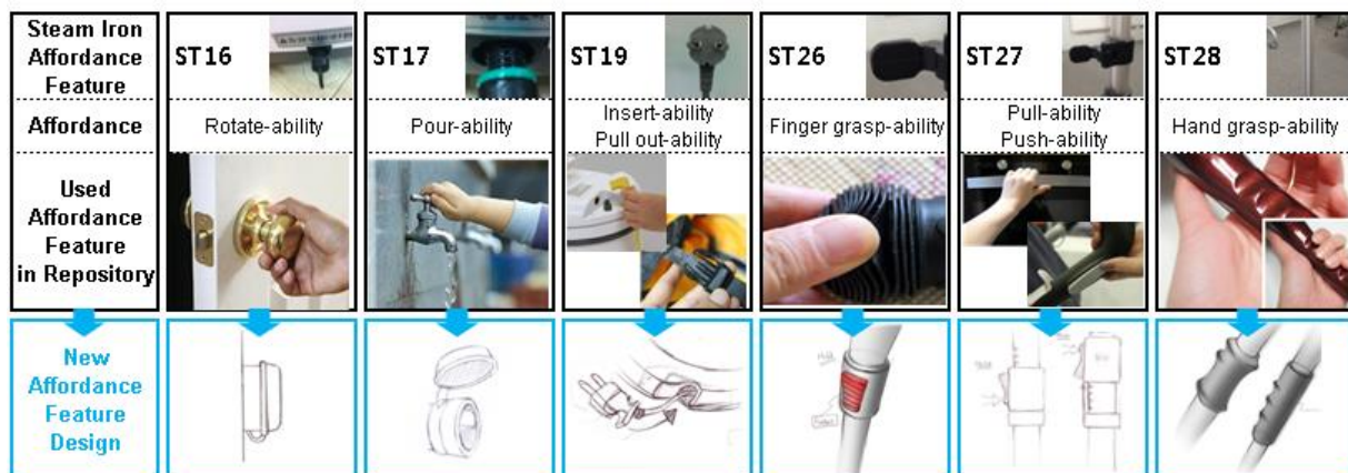
Figure 4. Using affordance repository new design of steam Iron
