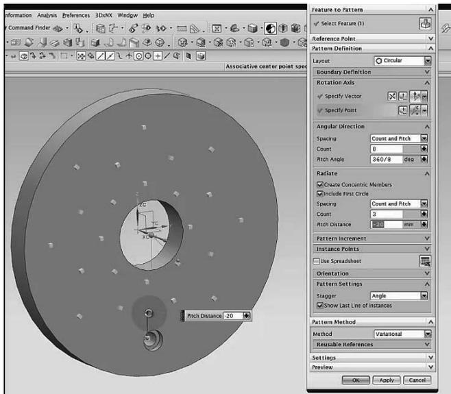
Figure 1. A screenshot showing how the video session shows actual work with the software, and illustrates points with arrows, markers, highlights and spoken explanations (example shows use of pattern feature for duplicating holes)
