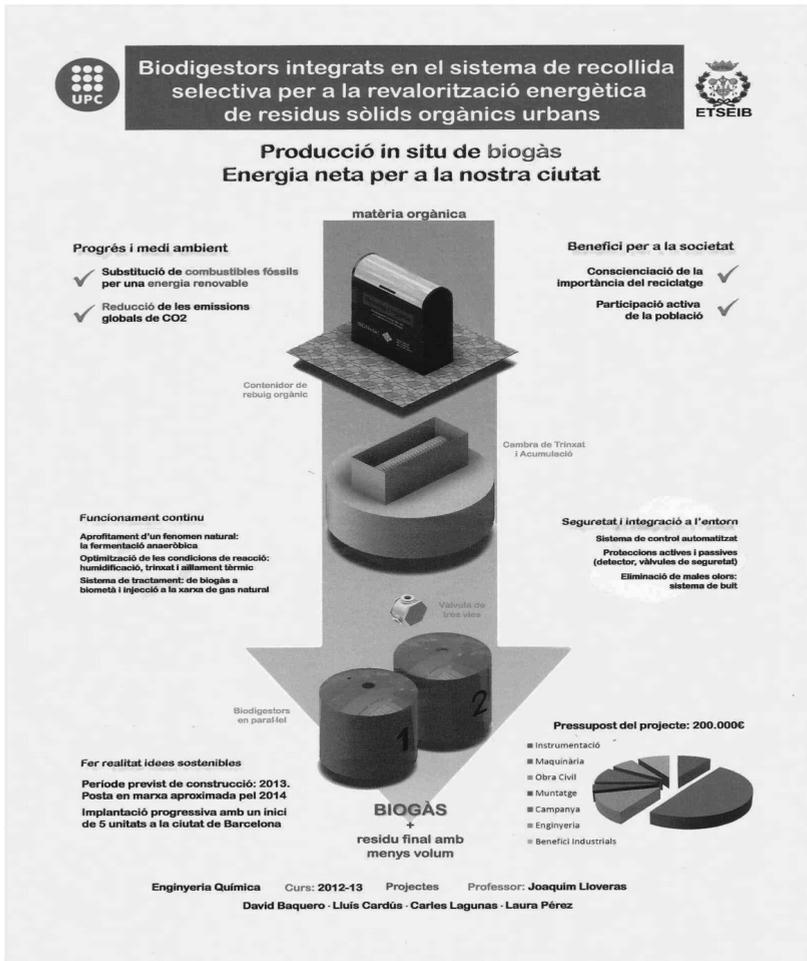
Figure 2. Poster of main parts of Biogas production system (Catalan)
