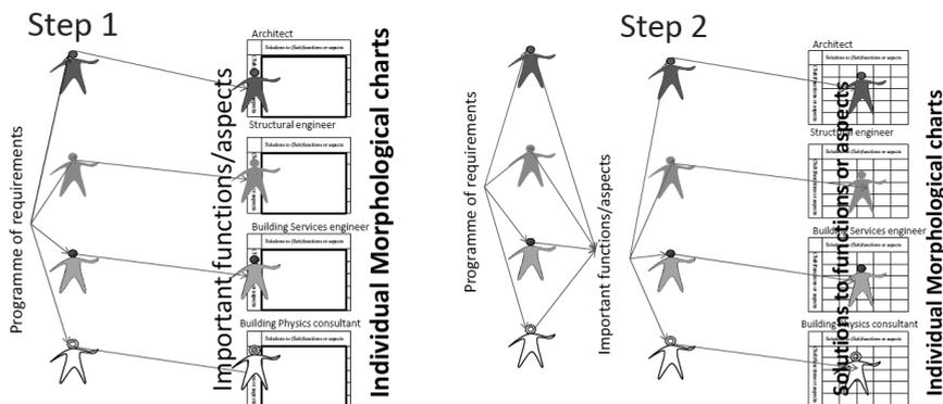
Figure 1. First two steps using the morphological charts in the Integral design method
