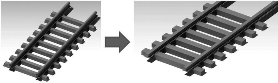
Figure 3. A piece of rail, optimized for design (left) and optimized for manufacturability (right)
