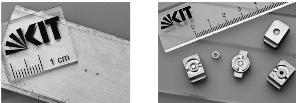
*Figure 1. Manufactured mold inserts during the CRC 499: gear wheels (left) and turbine wheels as well as bearing shields (right)*
