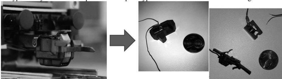
Figure 6. The task: a clutch for model railways (left) and the assembled prototypes (right).
