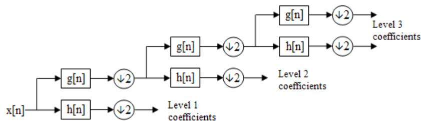
**Figure 1.** Three levels of decomposition of a signal using the DWT (taken from [http://en.wikipedia.org/wiki/Discrete\\_wavelet\\_transform](http://en.wikipedia.org/wiki/Discrete_wavelet_transform))
