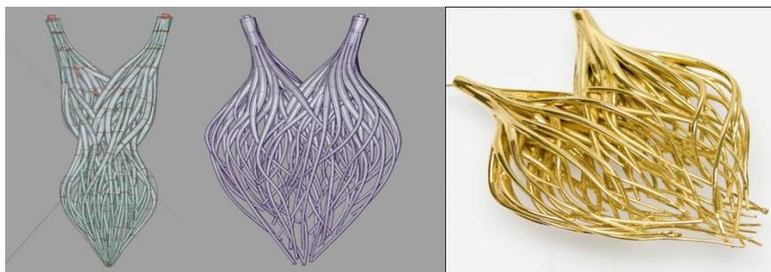
**Figure 3.** Manipulations of the Cuore design in CAD and the finished product in gold
