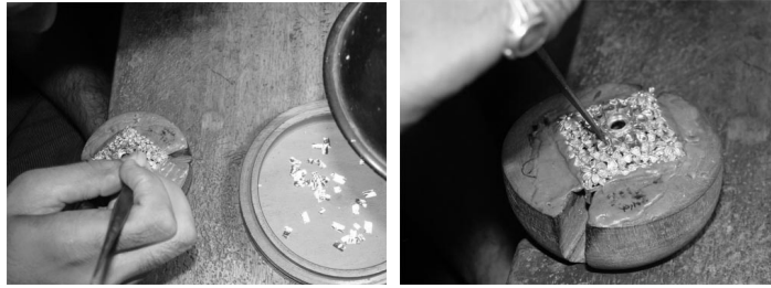
Figure 1. Gemstone setting using pliable gold foils. Source: Kundan workshop, Ahmedabad.
