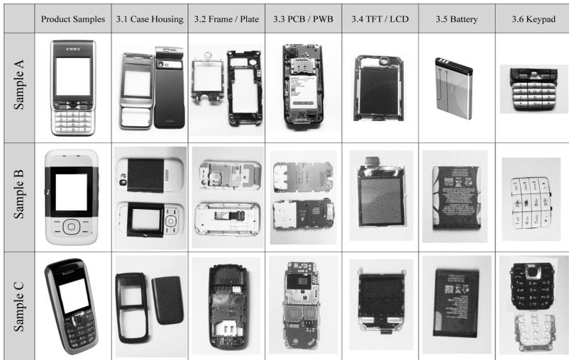
**Figure 3.** Product Sample Study of a mobile phone (Major modules of sample A, B and C)
