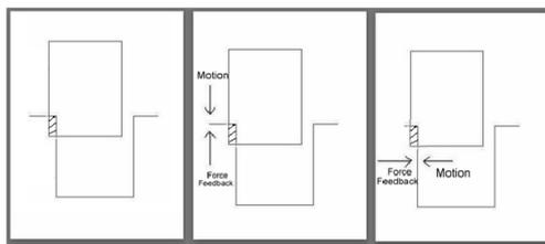
Figure 4. Different directions of force feedback for different directions of motion.
