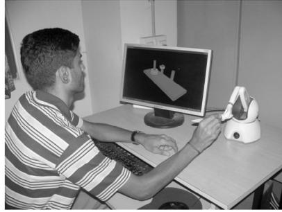
**Figure 5.** Towers of Hanoi using PHANTOM.
