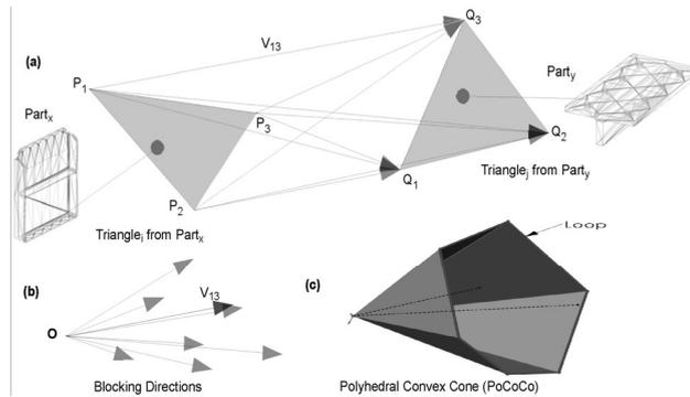
**Figure 1.** Computation of PoCoCo for a triangle pair.
