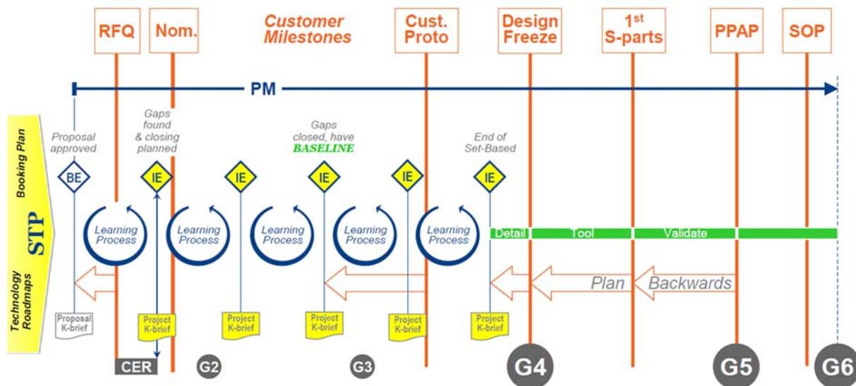
**Figure 5. An example of gate and milestone based product development model in car industry [Kongsberg Automotive 2010]**
