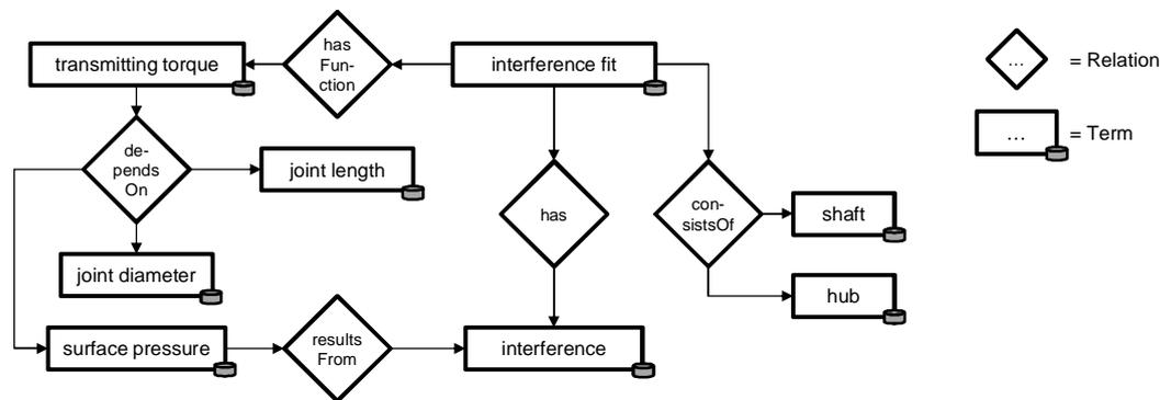
**Figure 4. A section of the semantic network in the domain of interference fits**
