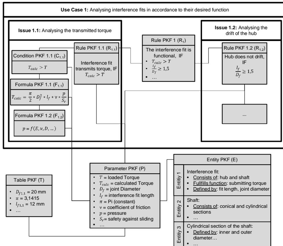
**Figure 6. Representation of exemplary use cases and issues considering Design for Function (DfF) and interference fits**
