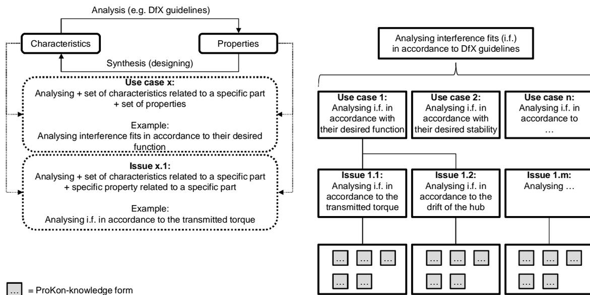
**Figure 5. Deriving the content of use cases and issues by using the CPM approach considering interference fits**
