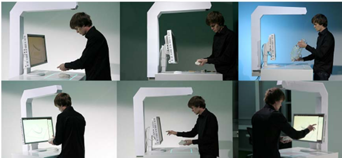
Figure 2. User interaction physical (top row) and virtual (below) with RSFF hybrid design tool
