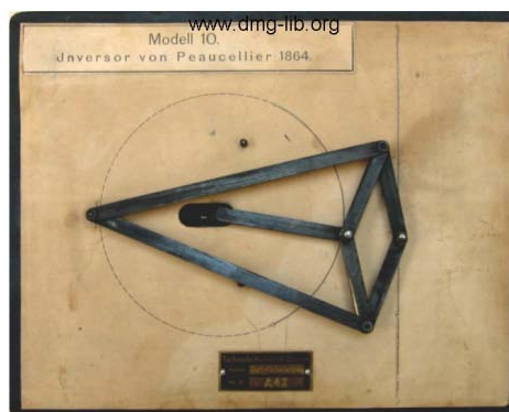
Figure 10. Photo of a model of a Peaucellier–Lipkin inversor on which the metadata description in Figs. 11 to 14 is based on
