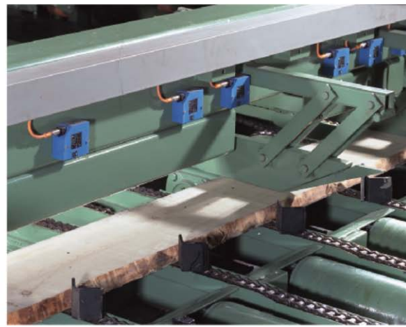
laser scanner for board wane detection
