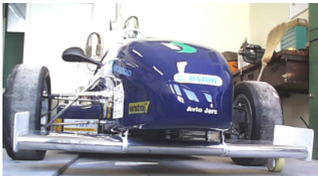
Figure 7. Front wing design
