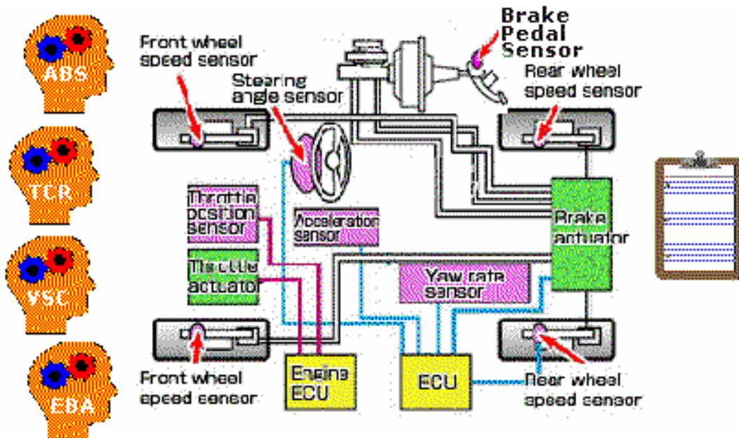
Figure 3. Active safety systems' organs structure. Active safety systems are an example of distributed architecture
