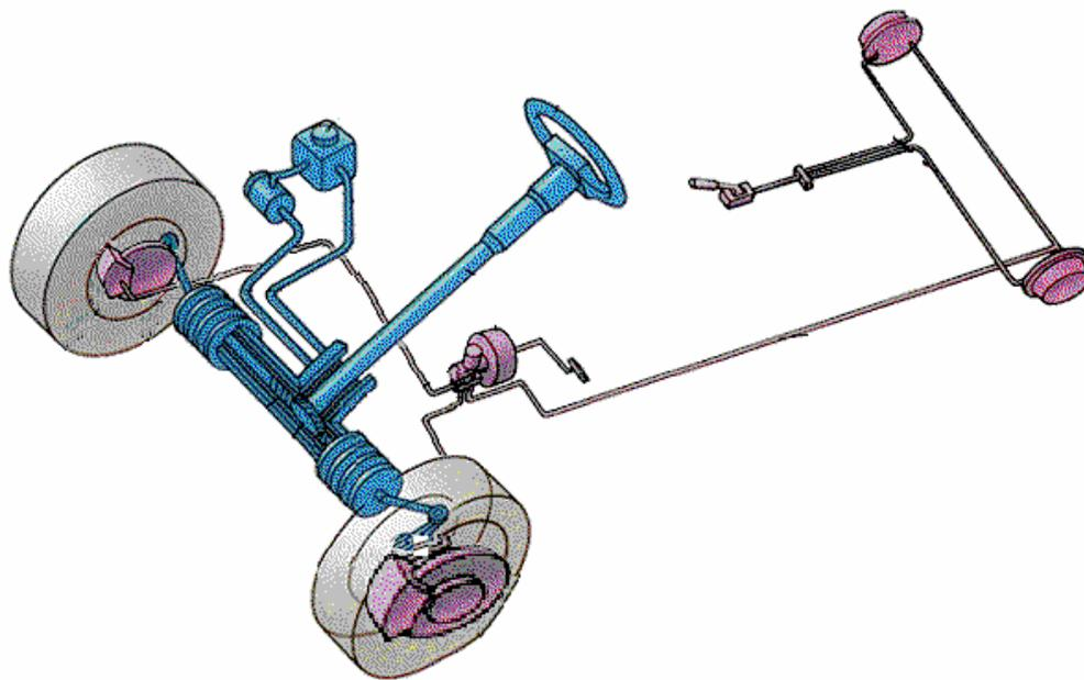
**Figure 5. The brake and steering chassis system. The brake and steering system is an example of mixed architecture**
