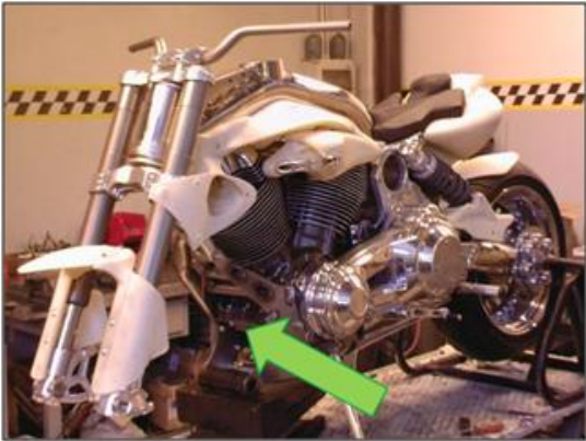
Figure 18a. Oil heat exchanger housing
