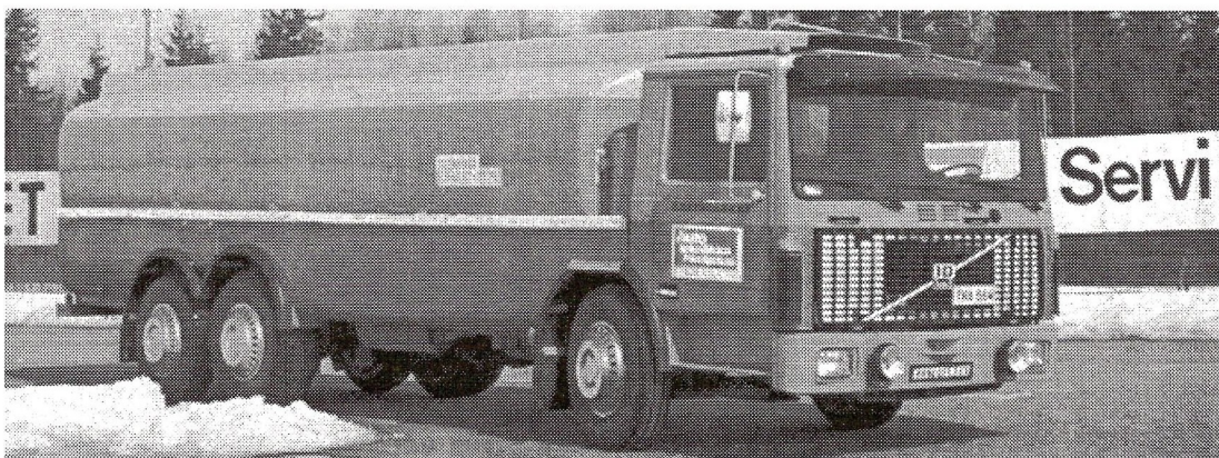
Figure 5. In some product areas modular product structures are used successful and almost without difficulty. One such product area is highway truck. It seems to be due the fact that customer's idea of functional structure is similar to assembly structure. For example Finnish-made self-supporting aluminium tank truck was not accepted by market, which expected separate chassis. So despite unequalled weight/load ratio (20 % increase in payload!) and superb riding qualities, the Hollming-truck flopped in the market.
