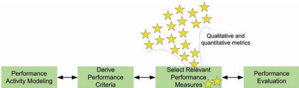
Figure 3. Four steps to accomplish performance evaluation to support the actual work that is being performed in product development.
