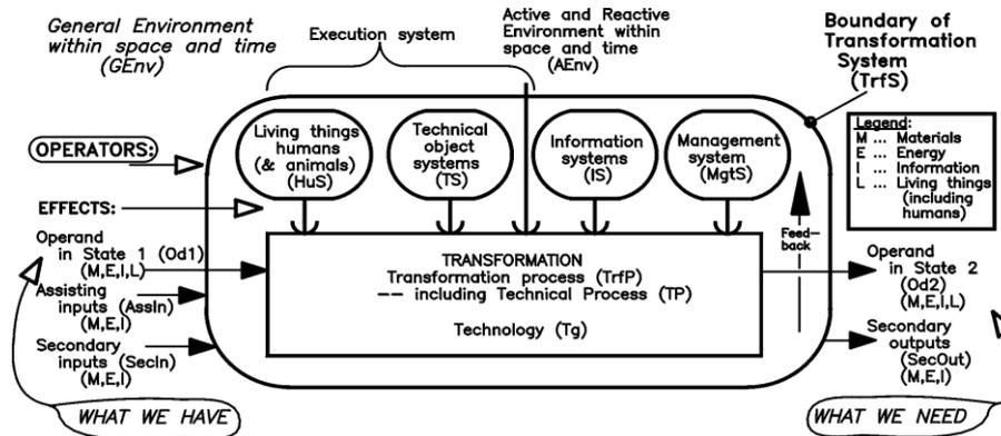
Figure 1. General Model of a Transformation System [1]
