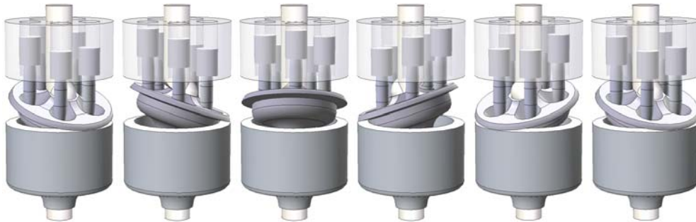
Figure 2. The motion of the expander illustrated in a series of snapshots over one engine shaft revolution.
