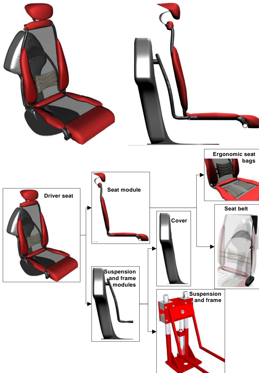
Figure 8. The driver's seat concept and its main modules (Henriksson et al. [11])
