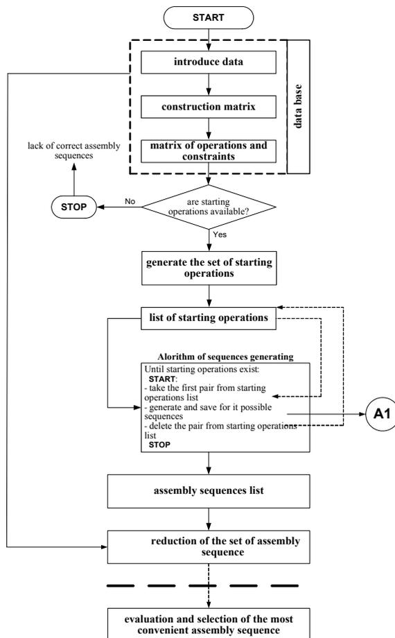
Fig.5. Algorithm of assembly sequence assignment
