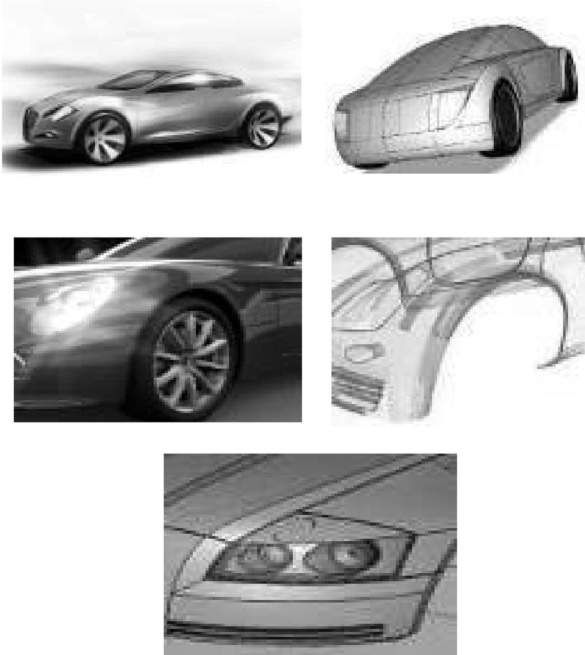
**Figure 6: Complete design workflow from concept sketch to technical surfacing**
