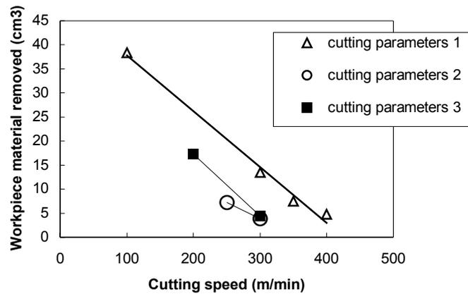
**Figure 4. Workpiece material removed for cutting parameters No.1, 2 and 3 as a function of cutting speed**
