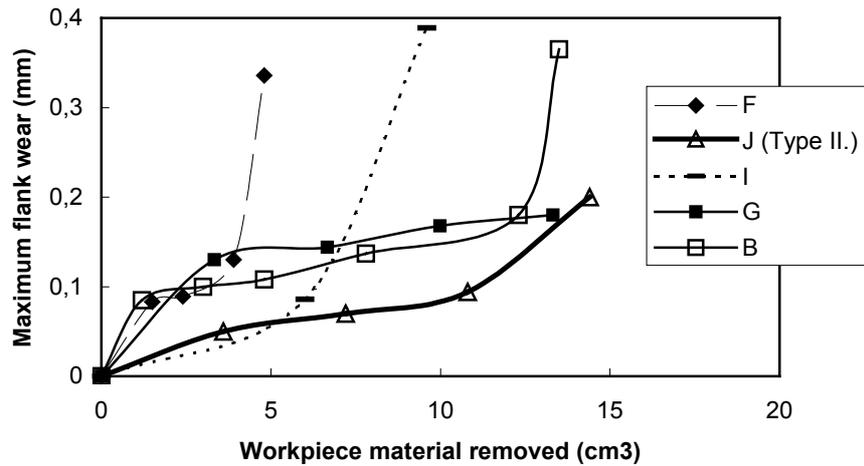
Figure 5. Maximum flank wear vs. tool life for different cutting parameters
