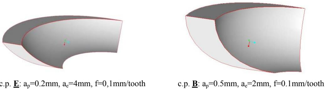
**Figure 3. Constant volume of the material removed per revolution with different cutting parameters set**
