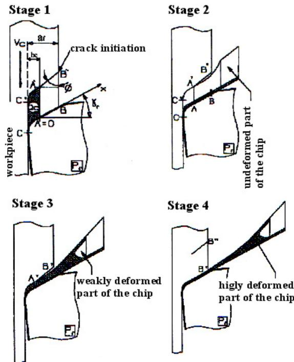
Figure 2. The different stages of segmented chip formation in HSC [4]
