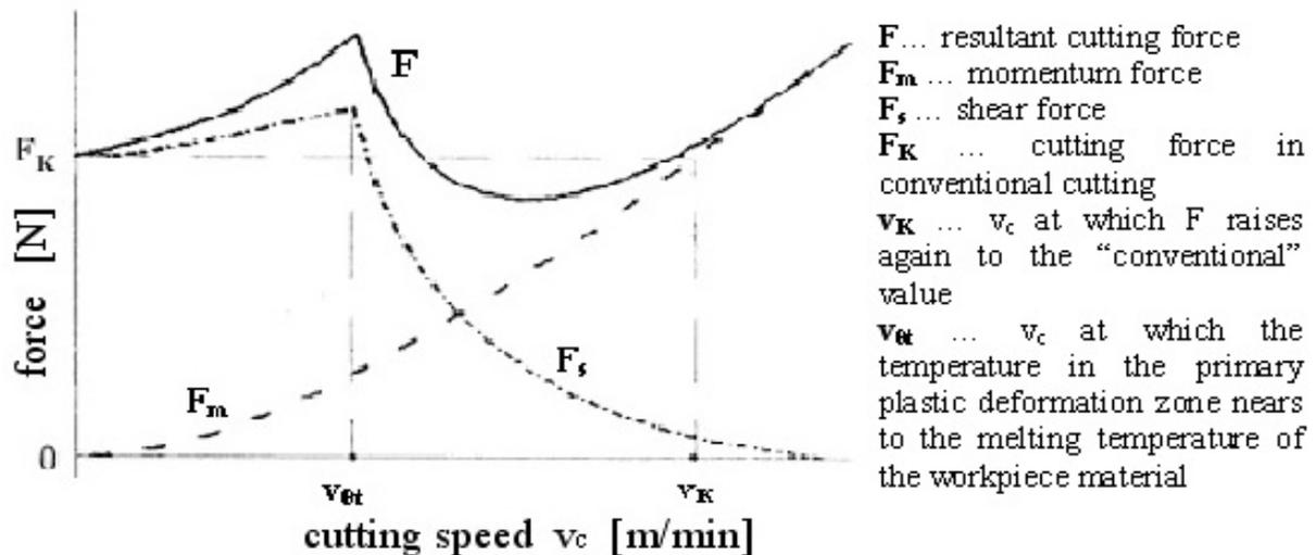
Figure 1. Theoretical behaviour of the resultant cutting force and its components v. cutting speed
