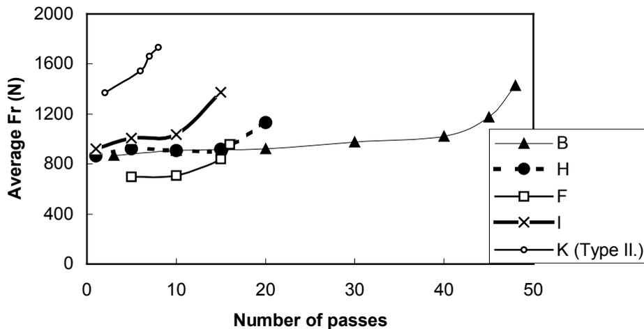
Figure 6. Effect of different cutting parameters on average milling force  $F_r$
