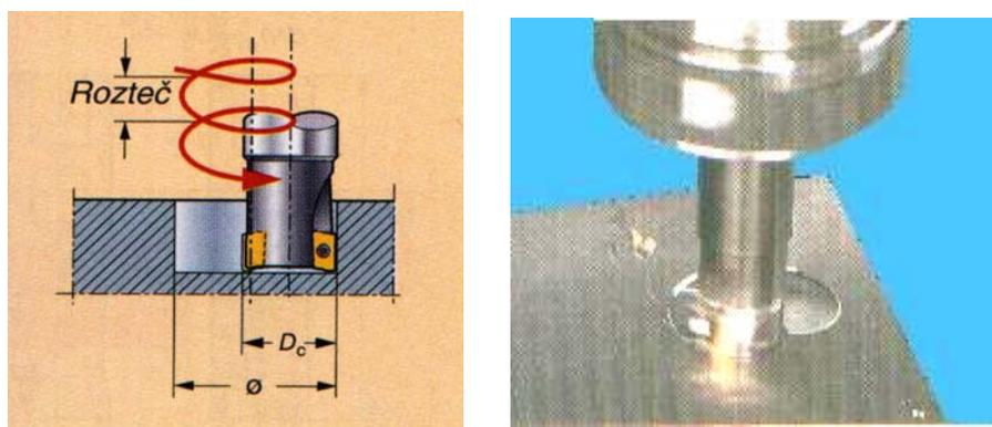
**Figure 14. Milling of a hole using a helix interpolation**
