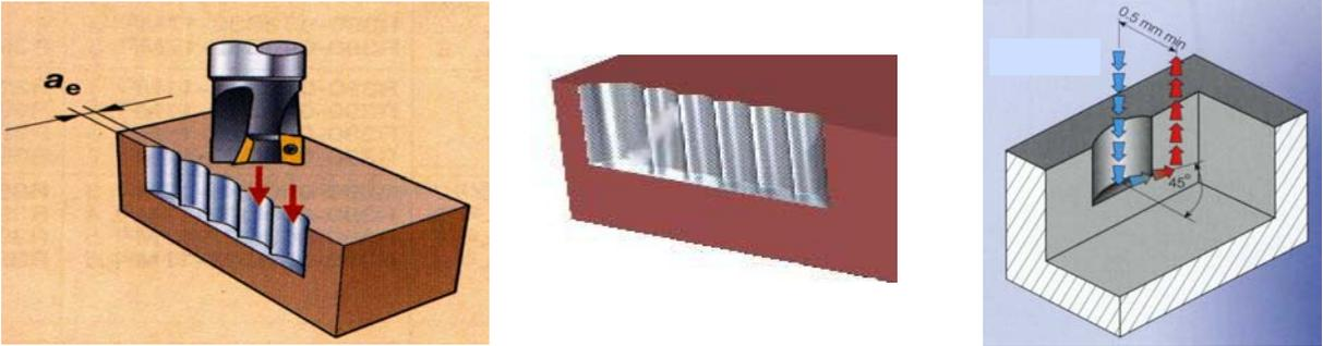
**Fig. 16 Grooving milling**
