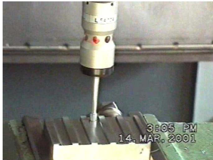
**Figure 13. Slot width measuring by a contact probe**
