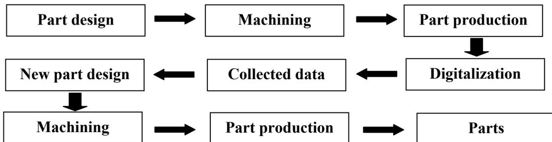
**Figure 7. Shape and dimension checking procedure**
