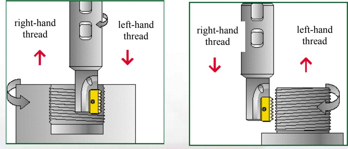
**Fig. 15 Milling of internal and external threads**
