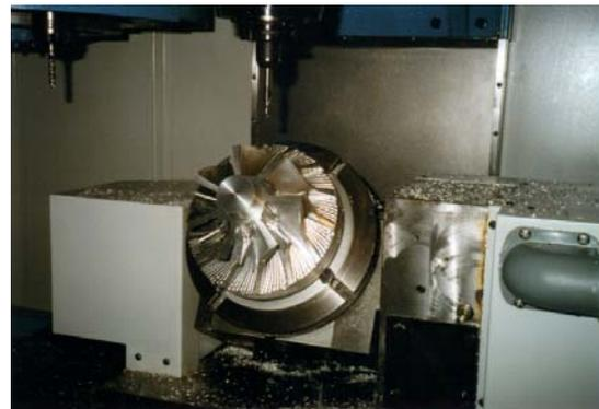
**Figure 3. Milling of a rotary wheel of a radial Turbo-compressor**
