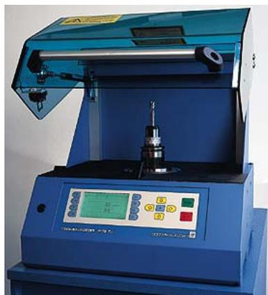
**Fig. 12 Balancing machine PTB – 7.1**
