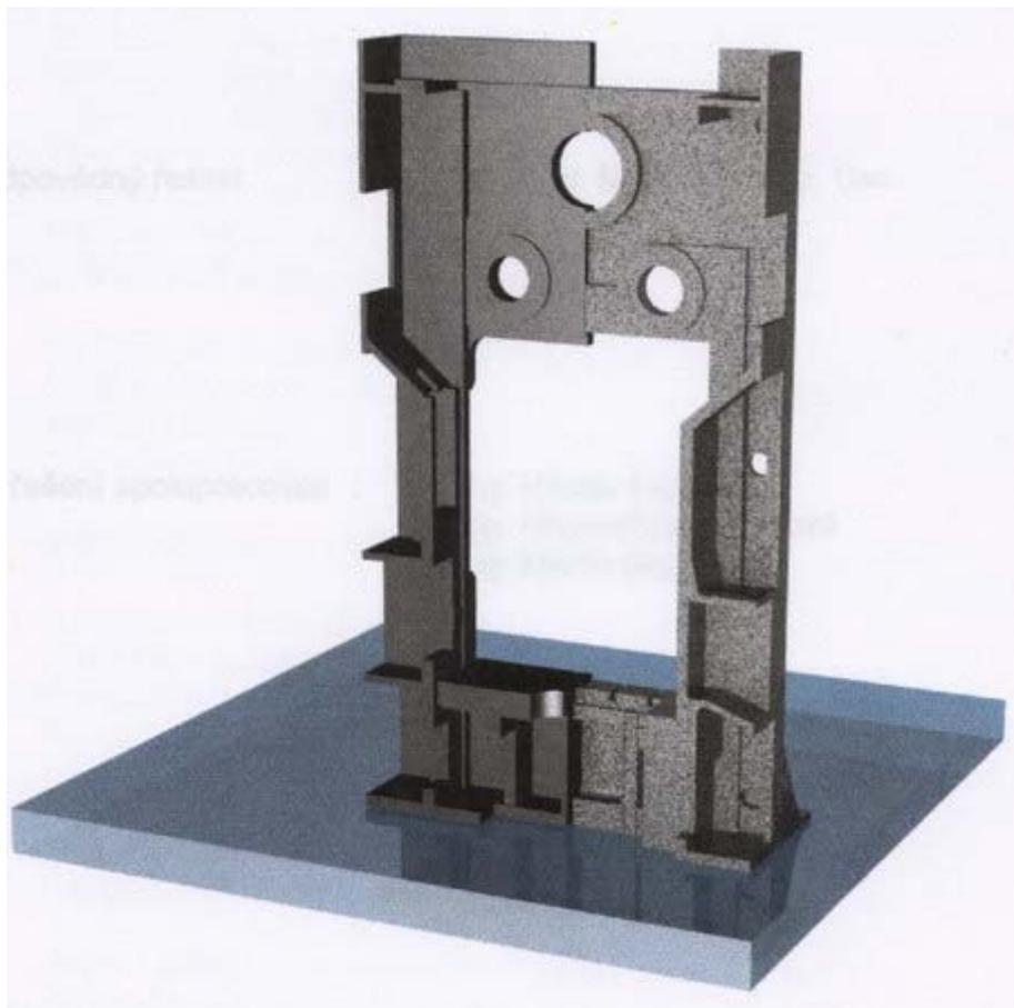
**Figure 10. Frame of press LDO 500**
