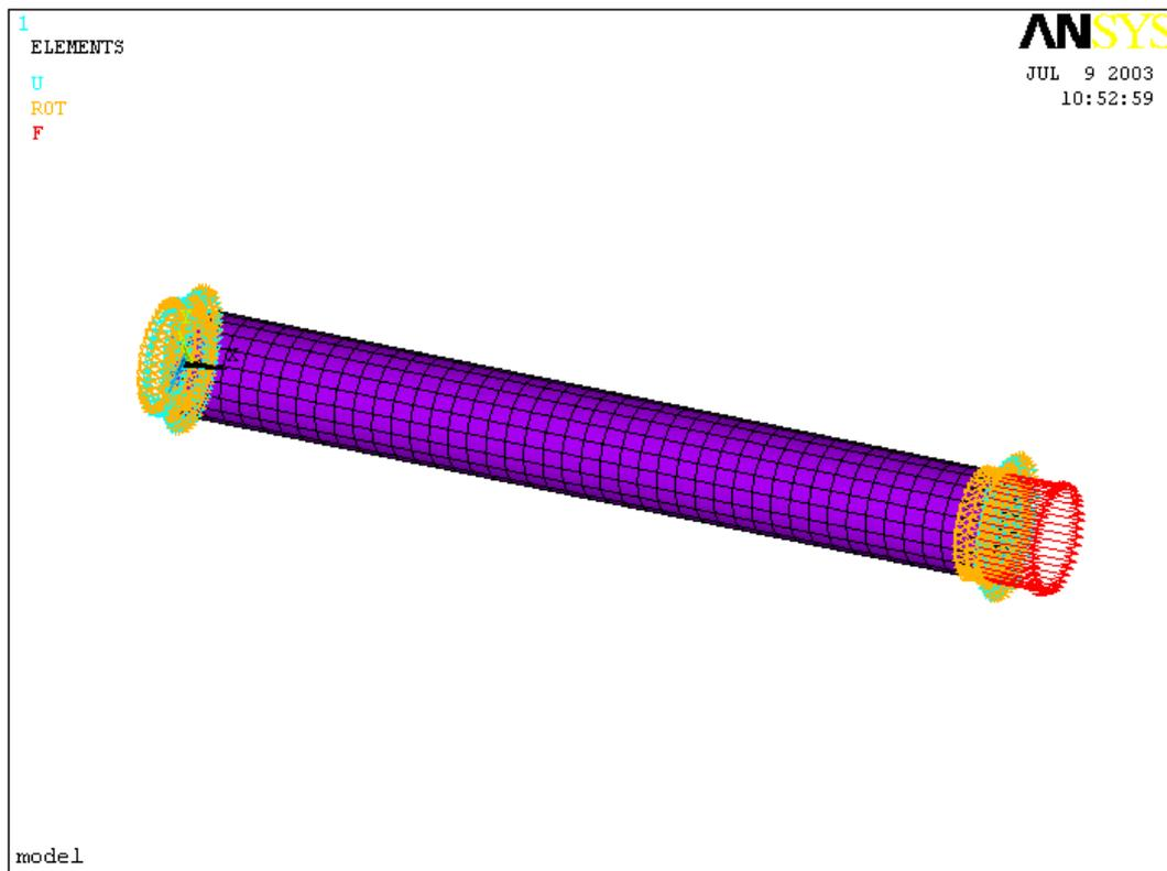
**Figure 3. One of the computational models with displayed boundary conditions**
