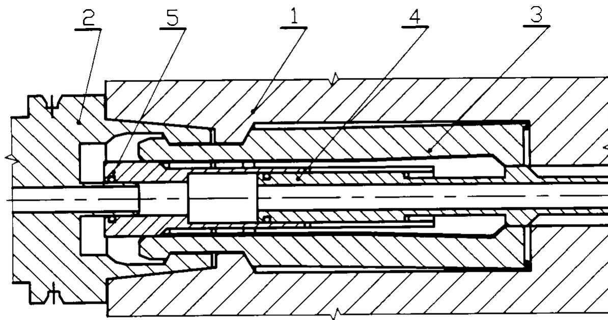
Figure 2. Tool clamping device for HSC – tool clamped
