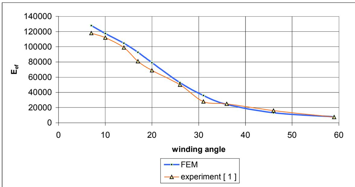
**Figure 6. Comparison of computed and measured effective modulus of elasticity in tension**
