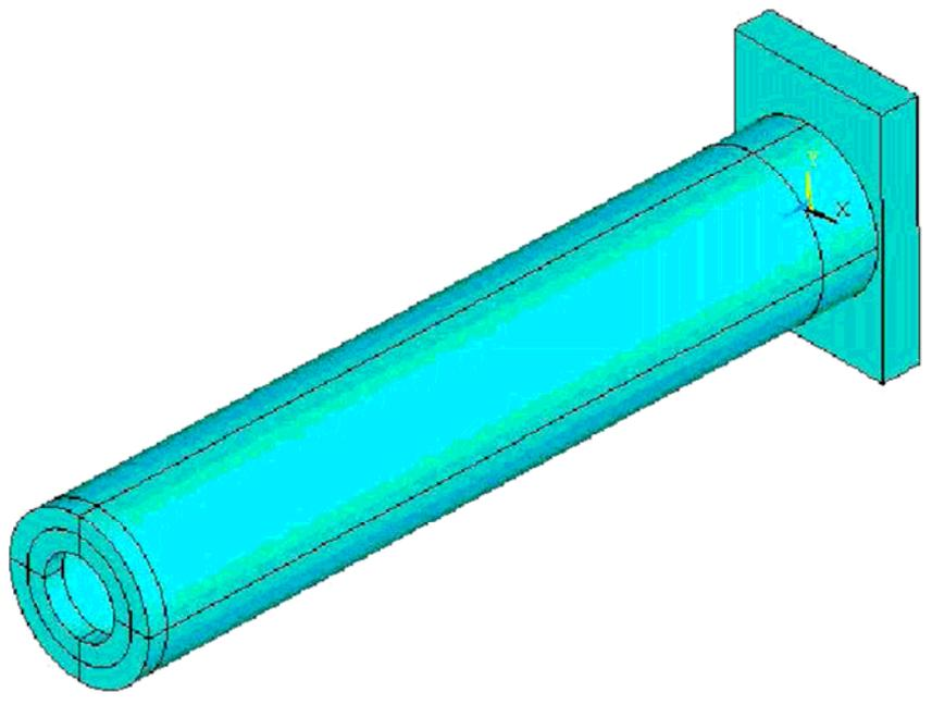
**Figure 9. Computational model of lengthening piece of milling equipment**
