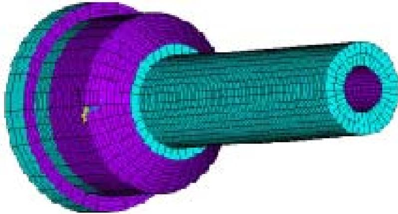
**Figure 8. Computational model of milling equipment body**
