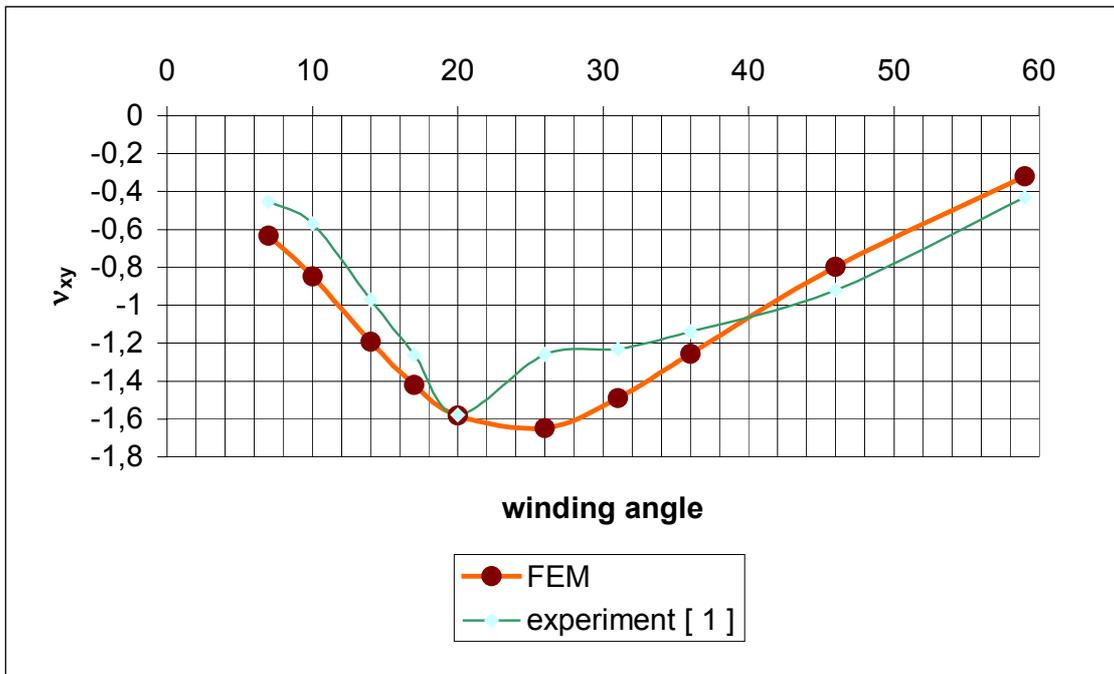
**Figure 5. Comparison of computed and measured effective Poisson's ratios**
