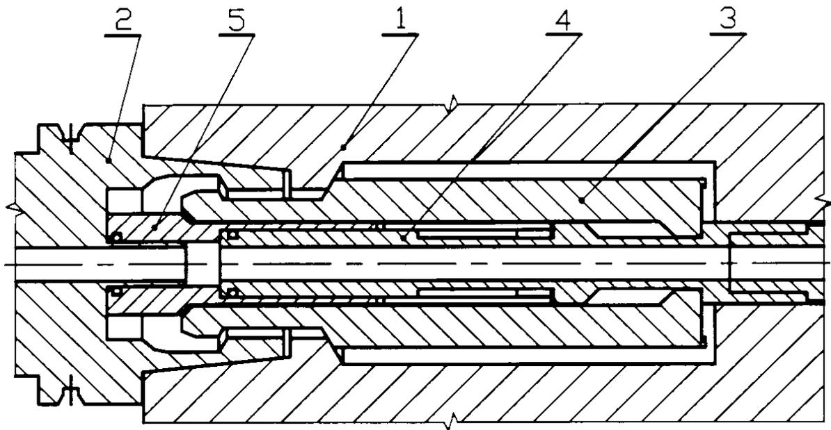
Legend: 1 – spindle, 2 – HSK clamping taper, 3 – gripping elements,
