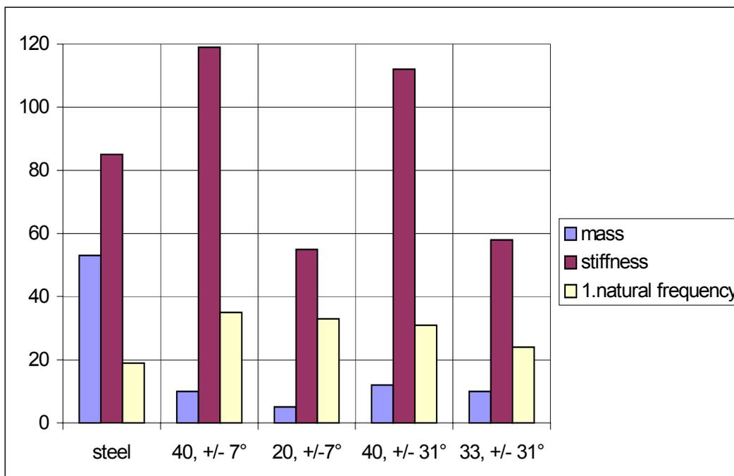
**Figure 7. Comparison of mass, stiffnesses and natural frequencies**
