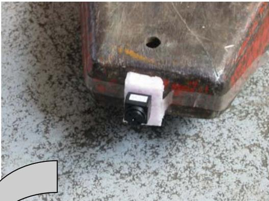
Figure 6. Camera on loading arm
