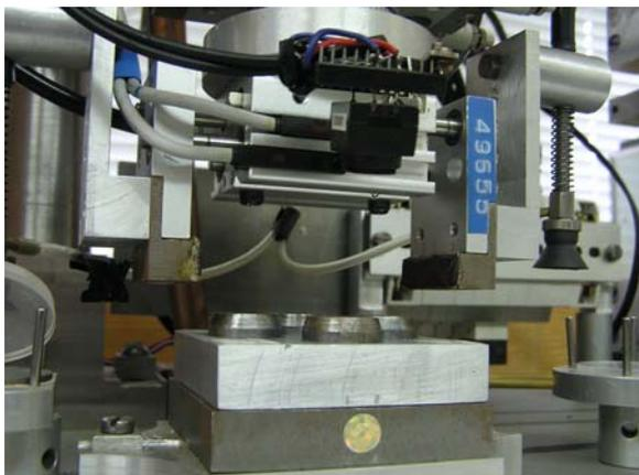
Figure 11. Camera module on the handling arm
