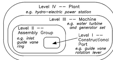
**Figure 2. Technical Systems Classified by Complexity**
