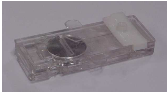
Figure 4. Early device assembled using injection moulded components
