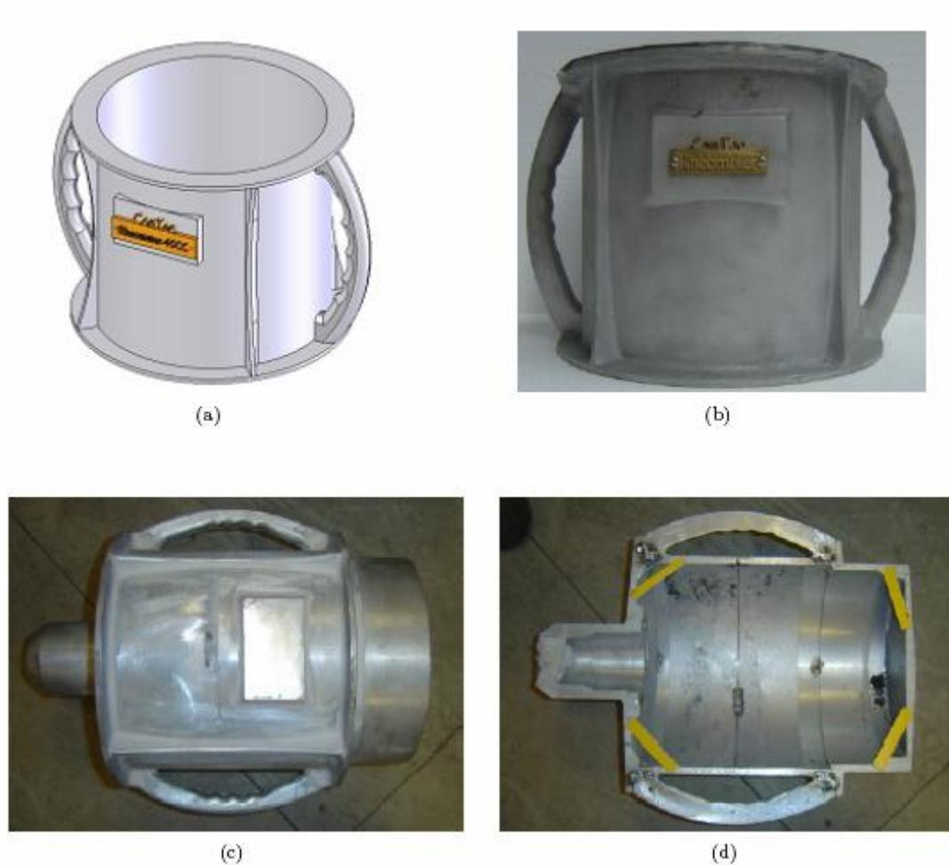
**Figure 2: Rheometer-4SCC sample bucket, CAD drawing (a), the final product casted out of aluminium (b), the outside of the mold (c) and the inside of the mold (d)**
