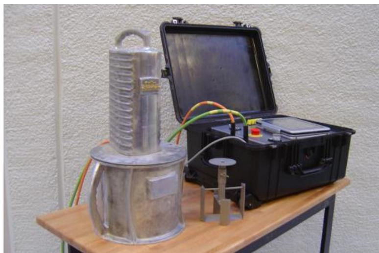
**Figure 3: Rheometer-4SCC prototype 2**
