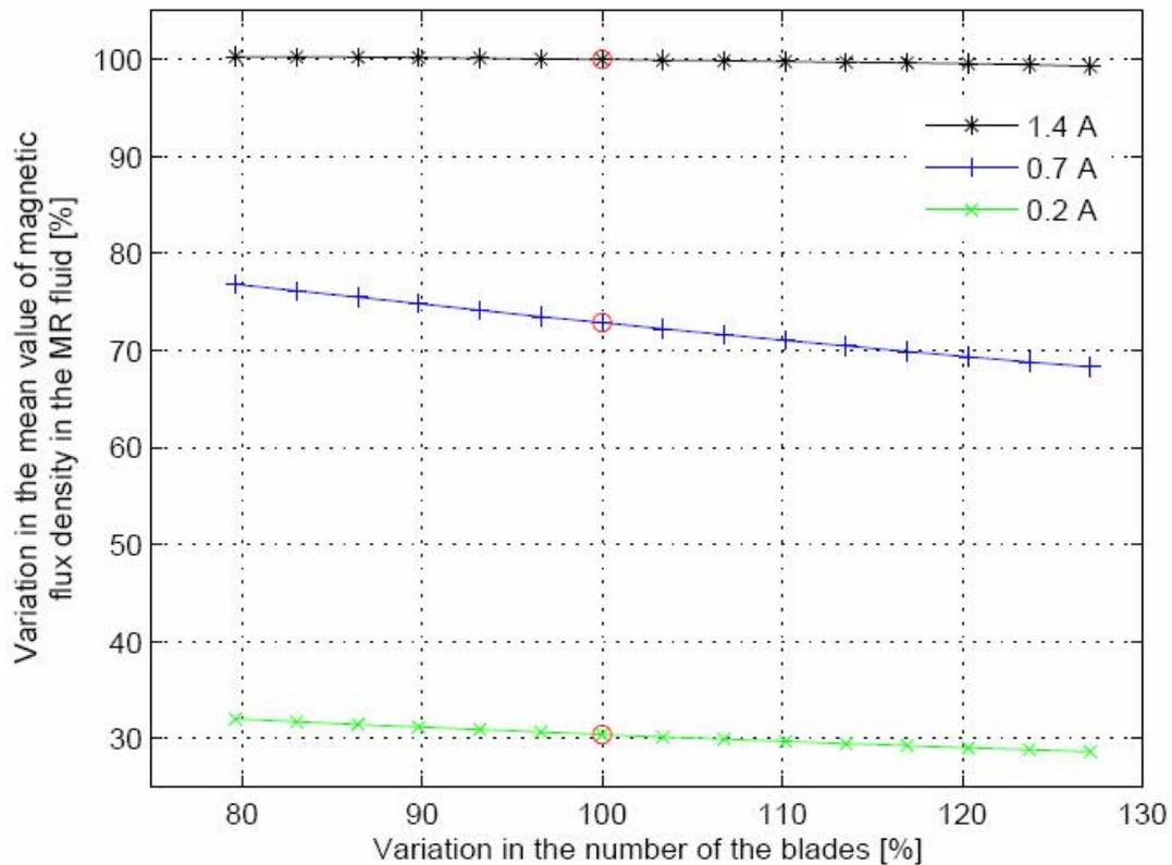
**Figure 5:** The variation in the mean value of the MFD in the MR fluid as a function of the variation in the number of the blades, for three values of the applied current: 1.4 A, 0.7 A, and 0.2 A. The red circles in the figure indicate the current working value.
