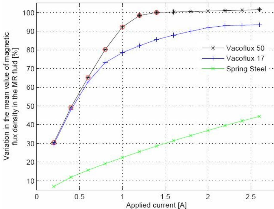
**Figure 4:** The variation in the mean value of the magnetic flux density in the MR fluid as a function of the applied current for three different materials in the core and the core sides. The materials are Vacoflux 50, Vacoflux 17, and Spring steel. The red circles in the figure show the values currently in use.
