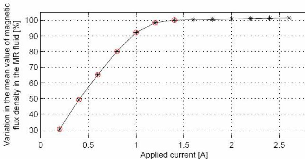
**Figure 3:** The variation in the mean value of the magnetic flux density in the MR fluid as a function of the applied current. The red circles in the figure denote the values currently in use.
