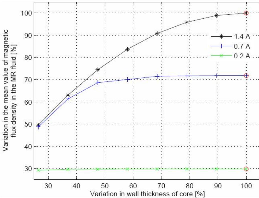
Figure 6: The variation in the mean value of the magnetic flux density in the MR fluid as a function of the variation in the wall thickness of the core, for three values of the applied current: 1.4 A, 0.7 A, and 0.2 A. The red circles in the figure show the value currently in use.
