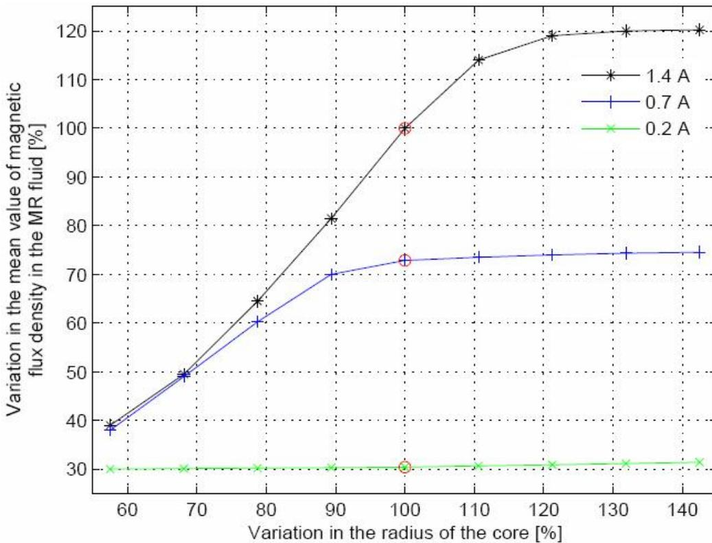
Figure 7: The variation in the mean value of the magnetic flux density in the MR fluid as a function of the variation in the radius of the core, for three values of the applied current: 1.4 A, 0.7 A, and 0.2 A. The current value used for the radius of the core is indicated with red circles in the figure.
