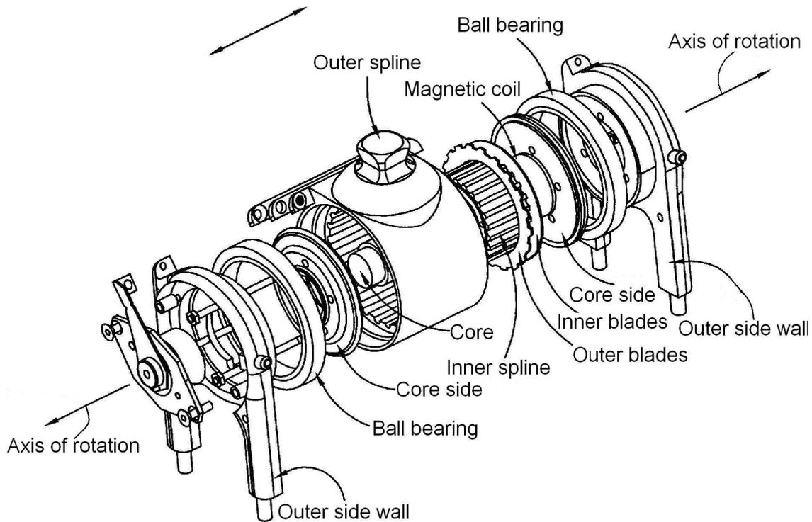
**Figure 1: A detailed exploded perspective view of a magnetorheologically actuated prosthetic knee [2].**
