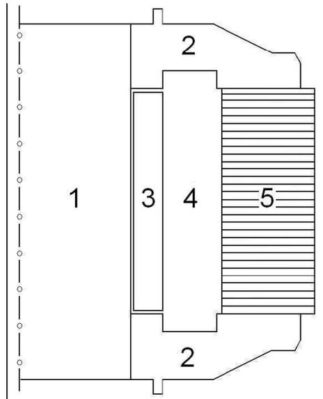
**Figure 2: A schematic of an axisymmetric finite element model. 1) the core, 2) the core sides, 3) the magnetic coil, 4) the inner spline, and 5) the blades with MR fluid thins between.**
