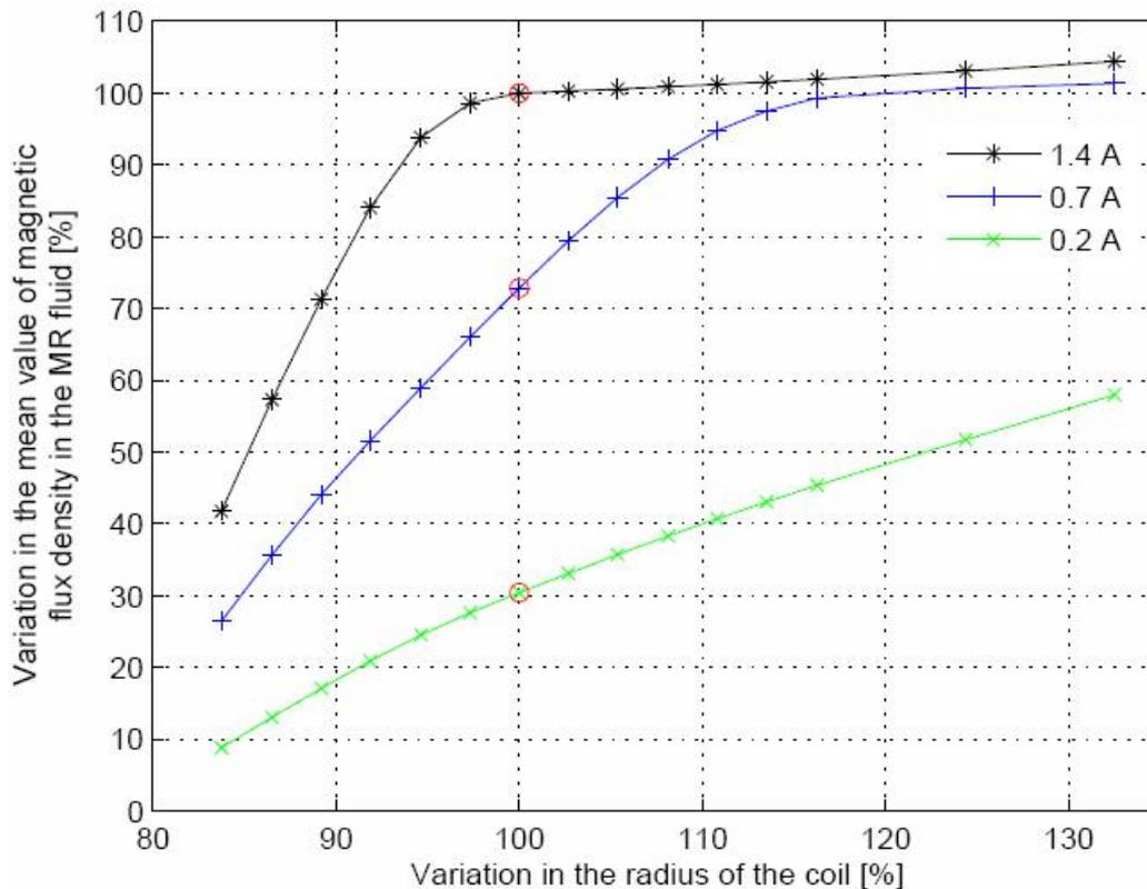
**Figure 8: The variation in the mean value of the magnetic flux density in the MR fluid as a function of the variation in the radius of the core without an external change, for three values of the applied current; 1.4 A, 0.7 A, and 0.2 A. The red circles in the figure show the current working value.**
