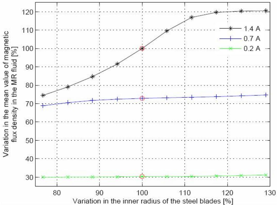
**Figure 9:** The variation in the mean value of the magnetic flux density in the MR fluid as a function of the variation in the inner radius of the blades without external change, for three values of the applied current: 1.4 A, 0.7 A and 0.2 A. The red circles in the figure show the current working value.
