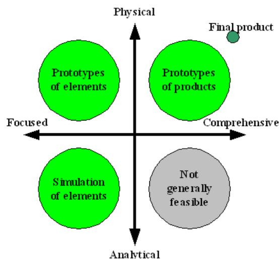
Figure 4 Classification of types of prototypes [13]
