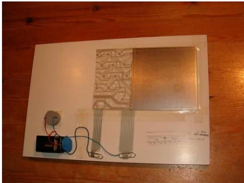
**Figure 7 The first sensi-touch model on aluminum.**
