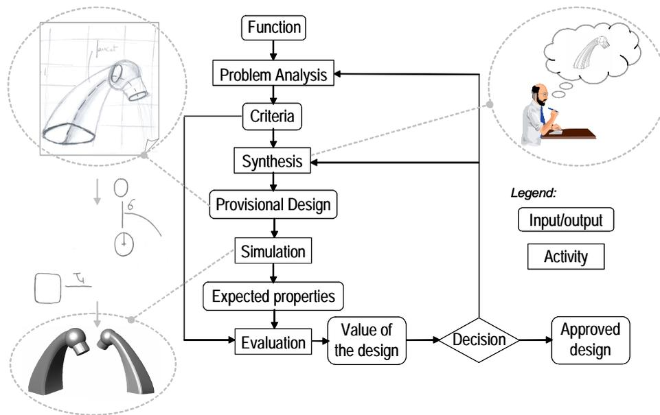
**Figure 6. Intended use of *PSL* in the basic design cycle**
