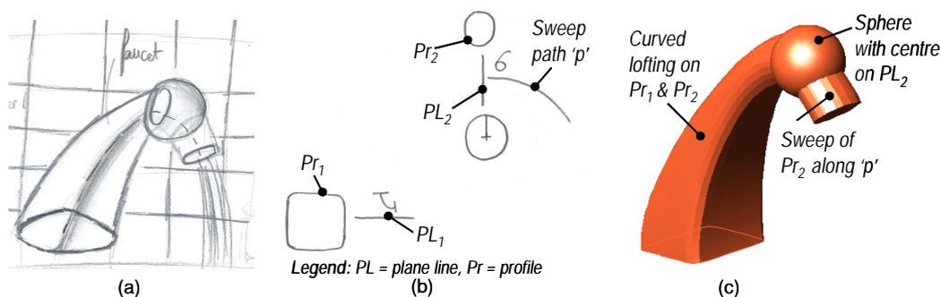
Figure 4. (a) Original scribble (b) representation of the faucet with PSL (c) 3D model generated
