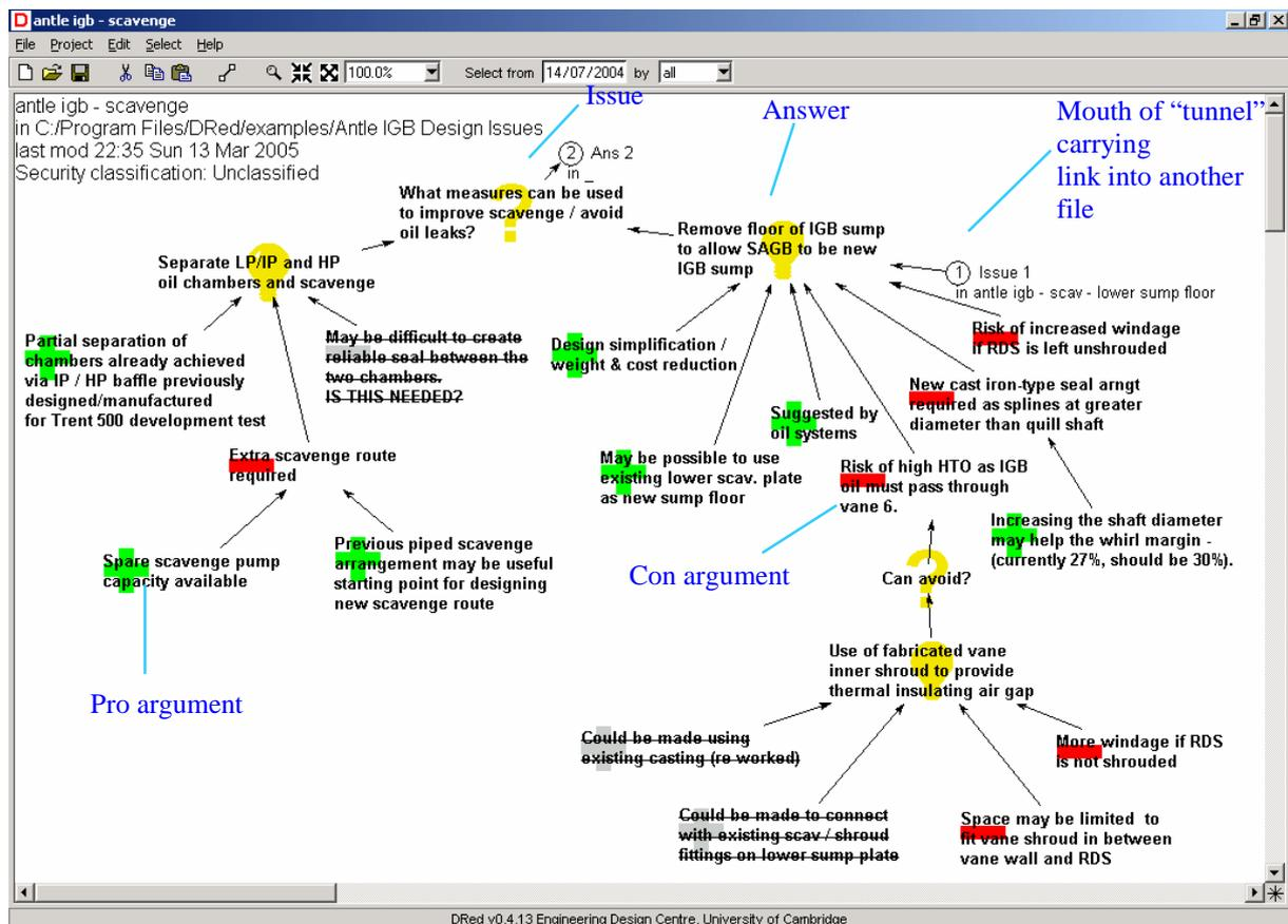
Figure 1. An example of DRed document capturing the design of an aero-engine internal gearbox
